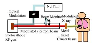
Figure 1: Concept of high performance IMRT, dynamic optical modulation of electron beam by a Photo cathode RF gun1
