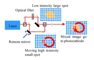
Figure 3: Basic experiment of dynamic optical modulation of electron beam.
