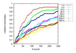
Figure 5: Beam-based IP position and IP angle feed-back simulation for the  $e^-e^-$  collision with ground motion model B applied during different times along the BDS. The average relative luminosity is calculated over 50 seeds.
