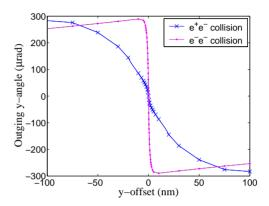
Figure 1: Vertical deflection angle versus vertical half beam-beam offset, for  $e^+e^-$  and  $e^-e^-$  collisions simulated with GUINEA-PIG [3], using ideal Gaussian beam distributions with ILC nominal parameters at 500 GeV in the center-of-mass [4].
