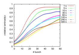
Figure 4: Beam-based IP position and IP angle feed-back simulation for the  $e^+e^-$  collision with ground motion model B applied during different times along the BDS. The average relative luminosity is calculated over 50 seeds.
