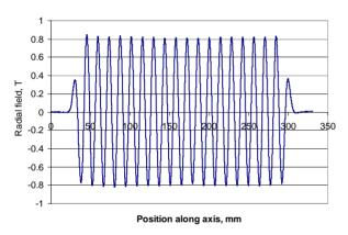
Figure 3: Profile of the axial component of the magnetic field on the undulator axis measured for prototype 1.
