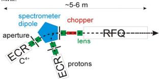
Figure 2: Schematic drawing of the beam injector scenario 2.
