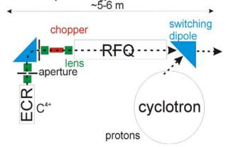
Figure 1: Schematic drawing of the beam injector scenario 1.
