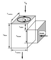
Figure 2. Model of heat transfer in liquid Li heated by a 40 MeV proton beam.
