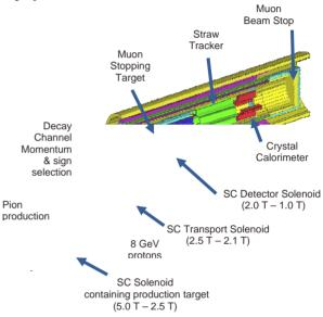
Figure 1: Conceptual picture of the MECO experiment at Brookhaven.
