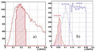
Figure 5: (a) A plot of the muon flux from the target produced by an 8 GeV proton beam and the subset (hatched area) that enters the first HCC segment. (b) A plot of the evolution of the muon momentum spread from the start of the cooling channel (z=0) through a series of HCC segments with reduced hydrogen absorber density to the stopping target at z=6.4 m.
