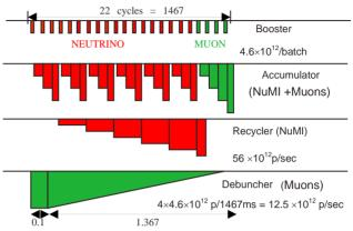
Figure 2: Potential Fermilab Proton source ring usage after the antiproton program ends.
