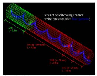
Figure 4: HCC with decreasing density used for first simulations.
