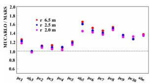
Figure 7: MUCARLO to MARS ratio for the number of muons at IR at various radii from the beam line for interaction of 250 GeV positrons with individual PCs and ABs.
