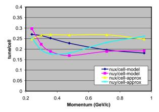
Figure 1. Dependence of cell tune on momentum in a nonscaling, linear-field FFAG which is tune-stabilized for medical therapy. In the legend, approx means the solution obtained from solving a set of approximated optical equations and model means the tune as modeled in MAD using these solutions.
