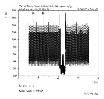
Figure 2: Beta-functions in the electron linac.
