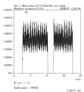
Figure 5: Vertical dispersion in the curved linac.
