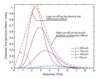
Figure 3: Predicted spectra (0.5 nC,  $\sigma_z=15~\mu m$ ,  $E_c=45~\text{MeV}$ ) of CTR collected by a 6-inch OAP (19° off-axis) for different plasma transverse boundary sizes ( $\rho$ ). The amount of emitted energy is strongly affected by the transverse boundary size of the emitting region.
