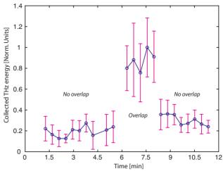
Figure 4: Enhancement (> 3) of the total amount of THz energy collected observed when the main pulse (acceleration) is preceded with a pre-ionizing beam (on/off experiment).
