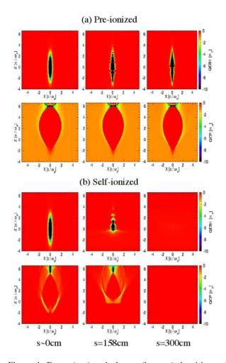
Figure 1. Beam (top) and plasma (bottom) densities at 3 different locations (s~0cm, 158cm and 300cm along the plasma) in (a) pre-ionized and (b) self-ionized plasmas
