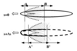
Figure 2. Schematic of the ionization front recession
