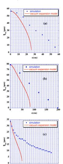
Figure 4. Ionization front location evolution for initial locations  $\xi_{i0}$  at (a)  $1.2 \sigma_z$  (b)  $1.7 \sigma_z$  and (c)  $2.2 \sigma_z$
