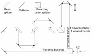
Figure 3. Laser configuration for the bunch train generation, consisting of 4 drive bunches and one witness bunch.
