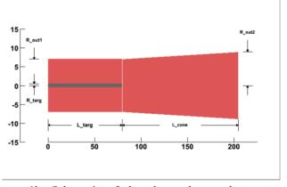
Figure 1b: Schematic of the plasma lens and target. Dimensions are given in cm.
