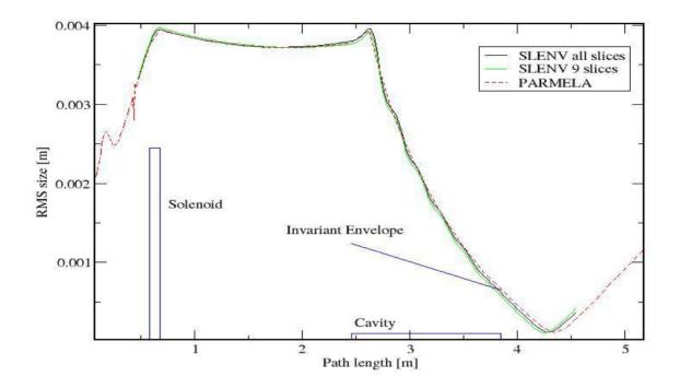
Figure 1: Beam Envelope calculated with PARMELA and SLENV
