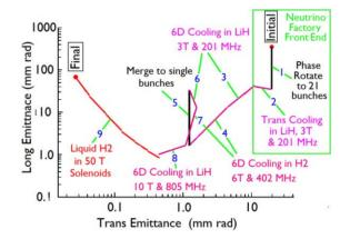
Figure 2: Transverse vs. longitudinal emittances before and after each stage
