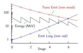
Figure 6: Results of ICOOL simulations of transverse cooling in liquid hydrogen in 7 sequential 50 T solenoids
