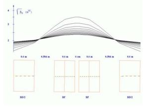
Figure 3: The horizontal betatron function in the "arc" cell.
