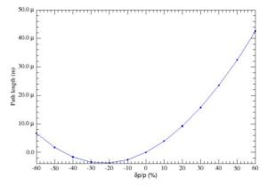
Figure 8: Path length dependence on momentum in the "IR" cell. (40µs corresponds to 0.133 ps).
