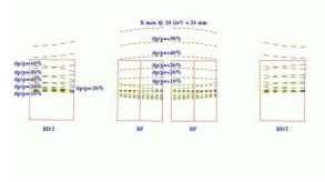
Figure 2: Magnets and orbit offsets in the "arc" cell.
