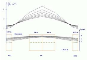
Figure 4: The horizontal betatron function and dispersion in the "IR" cell together with 0.7 m long BD and 0.4 m BF.
