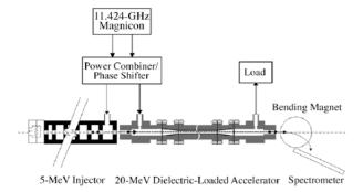
Figure 2: Schematic diagram of a dielectric-loaded test accelerator.
