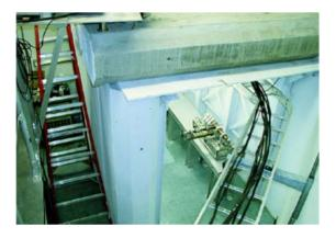
Figure 3: Photograph of concrete bunker, showing accelerator table and 5-MeV injector.
