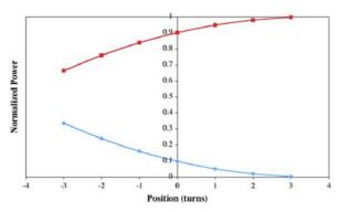
Figure 7: Normalized power into left and right output waveguides versus phase shifter position.
