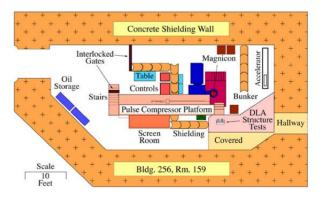
Figure 1: Floor plan of NRL Magnicon Facility.
