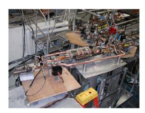
Figure 6: Photograph of power combiner assembly installed at magnicon output.
