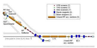
Figure 2: Layout of *LCLS* injector from gun to BC1.
