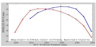
Figure 4: Measured effective field profile of center bends (dashed: <u>no</u> dispersion correction – solid <u>with</u> dispersion correction). The nominal BC1 position is 229 mm.
