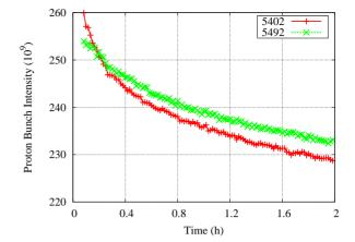
Figure 6: Intensity of the proton bunch no. 6 in the first two hours of a store. Store 5402 - before the correction of chromatic beta-function, store 5492 - after correction.
