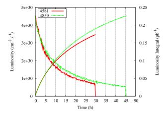
Figure 4: Single bunch luminosity and luminosity integral for stores 4581 and 4859.
