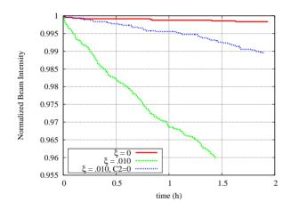
Figure 5: Normalized intensity of one proton bunch vs. time. Green line -  $\xi = 0.01$ , chromatic beta-function = -600. Blue line -  $\xi = 0.01$ , chromatic beta-function = 0. Red line -  $\xi = 0$ . Numerical simulation.
