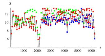
Figure 1: Radial beam separation at the collision helix in units of the beam size vs. azimuth starting from CDF IP. Blue - design helix, red - before installation of the new separators, green - present.
