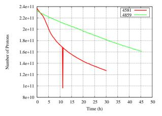
Figure 2: Single bunch proton intensity in two HEP stores. 4581 with the old helix, 4859 with the new helix.
