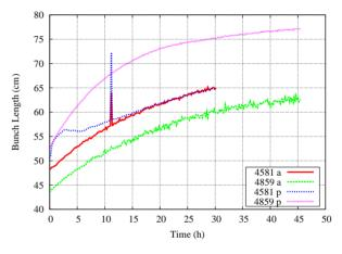
Figure 3: Proton and antiproton bunch length in two HEP stores. 4581 with the old helix, 4859 with the new helix.
