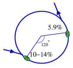
Figure 1: Locations of the partial snakes and the injection and extraction regions that give minimum polarization loss due to spin direction mismatch.
