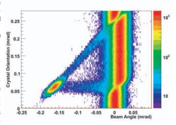
Figure 2: Angular scan of the ST4 crystal selecting only the middle horizontal part of the beam. On the ordinate axis the crystal rotation angle  $\phi$ ; on the abscissae axis the particle angle  $\theta$ .
