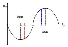
Figure 3: synchronous phases of a bunch leaving the accelerating structure and of a bunch that is injected into a decelerator.
