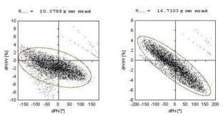
Figure 7: Output distribution with and without Debuncher.
