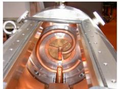
Figure 5: The Debuncher cavity before tuning and copperplating
