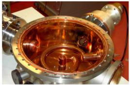
Figure 2: The Rebuncher-spiral-resonator with mounted plunger and coupling loop.
