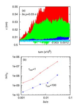
Figure 2: Emittance growth due to the fluctuation given by the strong-strong simulation.  $t_{cor}$  is the correlation time (turn) of the fluctuation.
