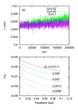
Figure 3: Evolutions of Dipole moment (a) and emittance (b) for various feedback gain with the kick noise  $\delta x = 0.02 \mu \text{m}$ . (0.12% of  $\sigma$ )
