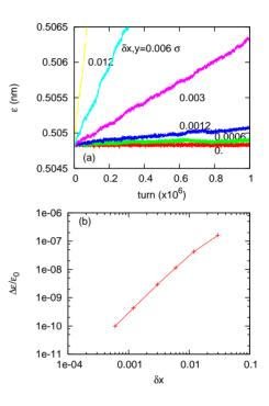
Figure 1: Emittance growth due to noise given by a weakstrong simulation. Plots (a) and (b) depict the evolutions of emittance for various noise amplitude and their emittance growth rate, respectively.
