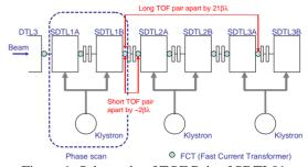
Figure 1: Schematic of TOF Pair of SDTL01.
