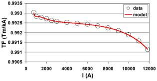
Figure 1: Average of the quadrupoles' main field (ramp up) measured and the static model fit with a max error equal to 0.01 units (measurement's uncertainty ~5 units for the transfer function).
