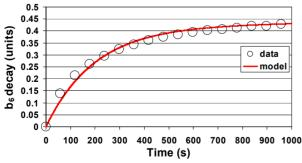
Figure 2: The decay of the b<sub>6</sub> of a main quadrupole at injection current plateau of 1000 s calculated with a standard pre-cycle.
