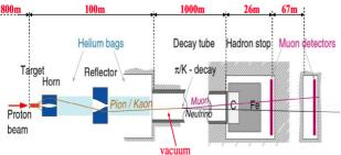
Figure 1: Main components of CNGS.
