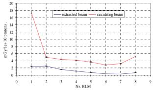
Figure 3: Beam loss per 10<sup>10</sup> protons for extracted (outside TPSG) and circulating (inside TPSG) beam.
