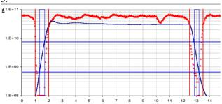
Figure 5: Measured particle distribution in red and kick waveform in blue.
