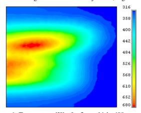
Figure 6: Temperature [K] of a 2 μm thick, 400 μg.cm<sup>-2</sup> graphite foil at the end of the injection of 7 CNGS pulses.
