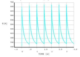
Figure 7: Peak foil temperature over 7 CNGS cycles.
