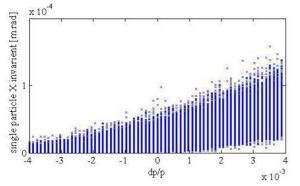
Figure 5: Horizontal single particle invariant (maximum amplitude) as a function of  $\delta p/p$  for CNGS beam.
