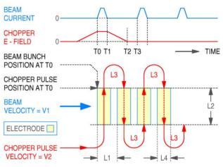
Figure 1: Slow-wave electrode design
