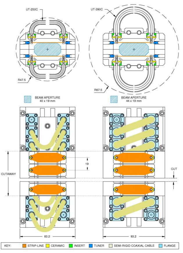
Figure 2: Electrode structures B1 and B2
