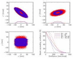
Figure 4: Phase space, Real space and Emittance occupancy of ISIS simulation at 0 ms with and without space charge.
