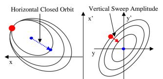
Figure 2: Phase space painting at Foil. Closed orbits in blue
