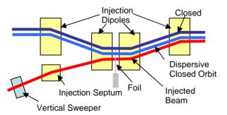
Figure 1: Schematic layout of ISIS injection system.
