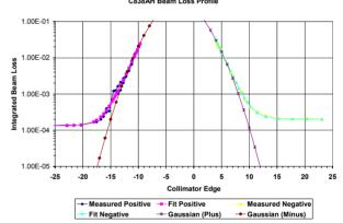
Figure 3: Integrated Beam Loss Profiles at C838A. Vertical profile show above and horizontal profile shown below. The data is shown with the exponential fit described in Table 2 and a Gaussian profile integrated from the beam edge on each side. Gaussian width adjusted to visually match halo data.
