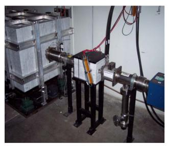
Figure 1: Collimator C836B, bellows, marble mask, Loss Monitor LM8C1 beside 836 marble mask with loss monitor LM8C3 above on wall, position monitor HP837, gradient magnet.
