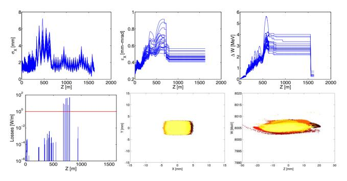
Figure 5: From top left to bottom right : RMS horizontal size, RMS horizontal normalized emittance, RMS energy spread, Beam losses, Transverse and Longitudinal distributions at the stripping foil. For a set of RF errors and magnetic field errors of  $(1\% 1^0 10^{-3})$  and a collimated beam of 45 mA.
