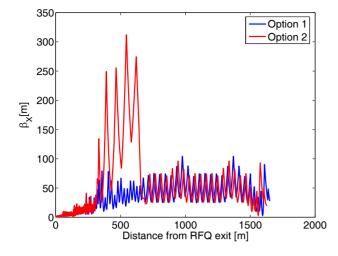
Figure 3: Horizontal beta function for the two options of the accelerator. Beam average current of 45 mA.
