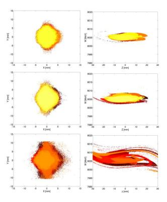
Figure 4: Transverse (left column) and longitudinal (right column) distributions at the stripping foil for 3 set of RF and magnetic field errors. First row :  $(0.5\% \ 0.5^0 \ 10^{-3})$ , second row :  $(1\% \ 1^0 \ 10^{-3})$  and third row :  $(2\% \ 2^0 \ 10^{-3})$ .
