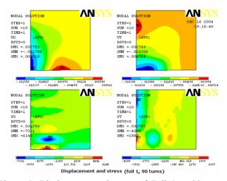
Figure 4: Displacement and stress of Foil 1 at 90-turn injection.
