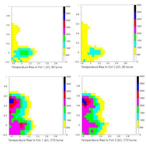
Figure 2: Temperature distribution from MARS: top -90-turn injection, bottom -270-turn injection, left - first foil, right - second foil.
