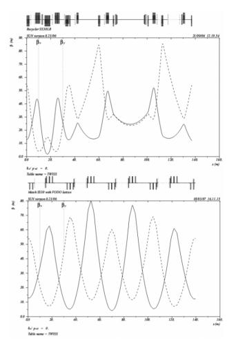
Fig.1 Beta-functions of existing SS30 for E-cool purposes (upper) and SS30-FODO with 3 quads in a half cell (lower).
