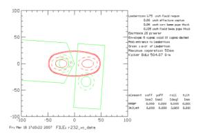
Fig. 5 The aperture at RR extraction Lambertson.
