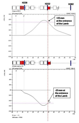
Fig. 4 Trajectories of circulating and extracted beam. The red blocks represent kicker modules. The blue blocks are 3 correctors.
