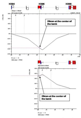
Fig. 6 The trajectories of the circulating beam (upper) and injected beam in Main Injector (down). The red blocks represent kicker modules. The blue blocks are 3 correctors.
