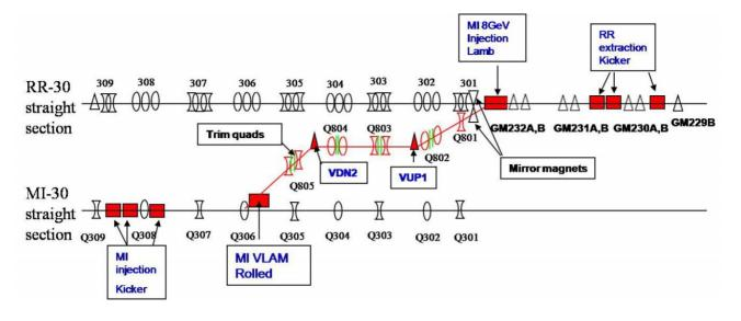
Fig. 2 Cartoon of extraction line, including RR and MI 30 straight section.
