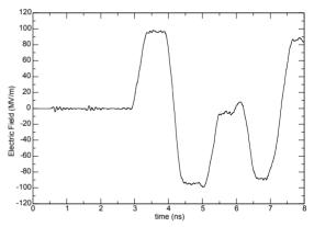
Figure 6: The on-axis time domain waveform in the middle of the structure shows the acceleration pulse for the proton bunch.
