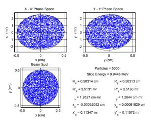
Figure 8: The result of accelerating a 0.78MeV 1cm dia. proton bunch through the structure using an acceleration schedule produces a well behaved phase space and beam spot size at the output of the 10cm radial stack. The beam gains  $\sim 9.2$ MeV of energy.
