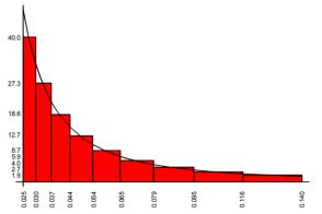
Figure 3: Adjusted relative permittivity profile versus radius (in meters) after the descretization process.
