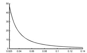
Figure 1: Using nominal values for the permittivity in the profiled radial line versus radius (in meters) given  $\varepsilon_{max} = 47.6$ , a = 25mm, and d = 1mm, yields Z(r)=0.347 $\Omega$ .
