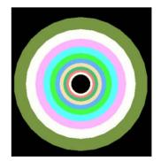
Figure 2: Typical radial grading process for discrete dielectric layers as used in the profiled radial line.
