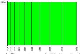
Figure 4: Time spent in each dielectric subsection showing the propagation time of the wavefront through the subsection vs. radius (in meters).
