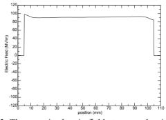
Figure 5: The on-axis electric field at a snapshot in time shows the uniformity of the field across the structure. Note that the two discontinuities are foils at the entrance and exit to the accelerator.
