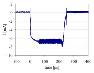
Figure 2: H- beam pulse ( $\sim$ 7 mA) as measured with ISTS Faraday cup. RF bunching voltage applied  $\sim$ 60 µs after the start of beam pulse and remaining on for  $\sim$ 400 µs.
