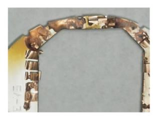
Figure 7: Damaged rf seal from a flex-flange connection.
