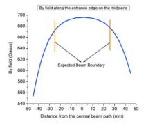
Fig. 3.4 Field distribution of the dipole along the entrance edges on the midplane.
