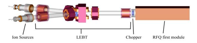
Fig. 1: Schematic Layout of the new magnetic LEBT for SNS power upgrade.
