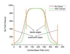
Fig. 3.3 Field distribution of the dipole along the central beam path on the midplane.
