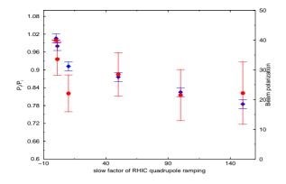
Figure 4: This plot shows the measured beam polarization after each resonance crossing as a function of the resonance crossing rate in units of RHIC qudrupole ramping slow factor. The higher the slowfactor, the longer it takes for the quadrupoles to ramp.
