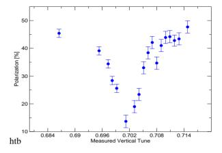
Figure 2: This plot shows the measured beam polarization as a function of the vertical betatron tune. The depolarization around  $Q_y = 0.7$  confirms the odd order snake resonance at  $Q_y = \frac{7}{10}$ .
