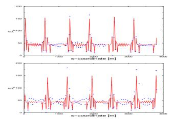
Figure 6: Measured RHIC injection optics with the new working points in Blue (top) and Yellow (bottom).
