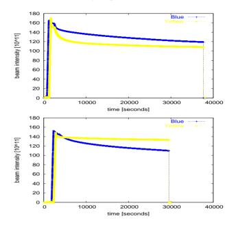
Figure 1: RHIC beam intensities during two stores in Run-6. In the top graph, tunes are set to (28.695, 29.685) in Blue and (28.685, 29.695) in Yellow. In the lower plot, tunes of the two rings are reversed.
