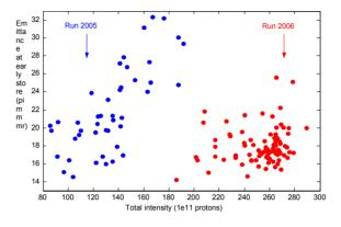
Fig. 1: Normalized beam emittance at early store verses total beam intensity in 2005 and 2006 100 GeV polarized proton runs.
