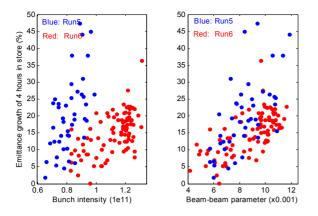
Fig. 6: The beam emittance growth of early 4 hours in store in Run 2005 and Run 2006 verses bunch intensity and beam-beam parameter.
