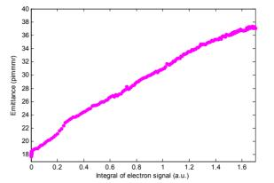
Fig. 8: Blue vertical beam emittance growth and the electron signal from the vertical electron detector at Blue section 1 in RHIC.
