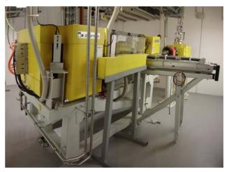
Figure 1: MLS RTM100 placed in the bunker with the movable fluorescence screen monitor (FOM) extension arm on the right side.
