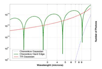
Figure 3: Hard edge/Gaussian beam Cherenkov coherent contributions. Gaussian TR is also showed
