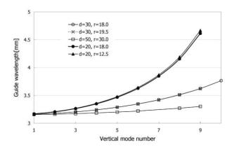
Figure 5: Guide wavelength of the W-band electromagnetic wave propagating in the quasioptical-resonator waveguide, shown as a function of the vertical mode number; m, of  $TE_{mn}$ , for various sizes.
