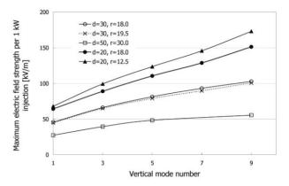
Figure 3: Electric field strength along electron beam axis as a function of the vertical mode number; m, of  $TE_{mn}$ , for various sizes.
