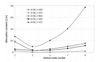
Figure 4: Attenuation constant of the W-band electromagnetic wave propagating in the quasioptical-resonator waveguide, shown as a function of the vertical mode number; m, of  $TE_{mn}$ , for various sizes.
