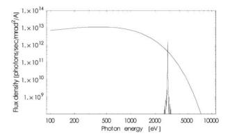
Figure 6: X-ray flux density of the undulator light. Synchrotron radiation from the bending magnet of TERAS is also shown in comparison.
