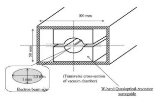
Figure 1: W-band quasioptical-resonator waveguide installed in the vacuum chamber of the storage ring TERAS of AIST.
