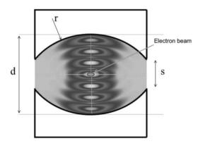
Figure 2: Electric field strength of  $TE_{70}$  mode calculated for W-band quasioptical-resonator waveguide. Radius of curvature; r, plate distance; d, and slit width; s are 18 mm, 20 mm, and 5 mm, respectively.
