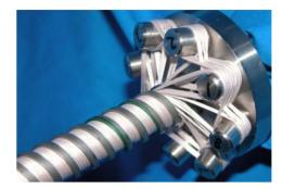
Figure 2: Undulator ends were designed for continuous winding of the double helix without any conductor joints. High-permeability steel poles were installed on the SS beam pipe before the coil winding.
