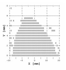
Figure 8. Dynamic aperture of Option 2, 400 turns.
