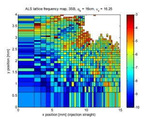
Figure 7. Frequency map calculated with realistic gradient and skew gradient machine errors, a vertical physical aperture of 4 mm and optimized settings for the additional sextupole families. The color code indicates diffusion rates on a logarithmic scale.
