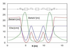
Figure 3. Optics of the Low Emittance Mode
