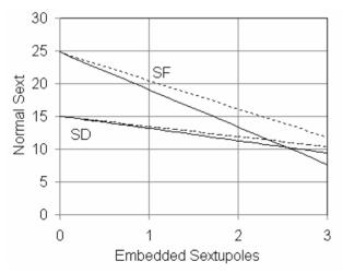
Figure 5. Reduction of normal sextupole strengths for chromaticity correction in presence of embedded sextupoles. Solid lines are for Option 1, and dotted for 2. The values are integrated K values [T/m].
