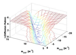
Figure 6. Sum of all frequency map diffusion rates for 500 initial conditions versus the strength of the 2 additional sextupole families. One can see a fairly extended area of small diffusion rates with a broad minimum.
