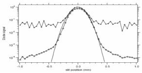
Fig. 5. Measured horizontal profile at BL 5.3.1 at 5 keV. The crosses and circles represent two amplifier gains and the line without symbols shows a Gaussian fit (Data provided by Robert Schoenlein).
