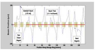
Fig. 1. Orbit Change for a One Kicker Magnet.
