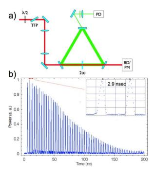
Figure 2: (a) RING cavity experimental set-up and (b) the associated recirculating  $2\omega$  signal in the cavity vs time. The integrated energy is  $28.5 \times$  higher than for a single pass. The temporal pulse separation of 2.9 nsec shown in the inset corresponds to the roundtrip time of the cavity.
