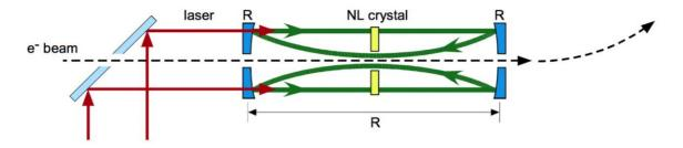
Figure 4: RING cavity design for Compton-backscattering based light source. The entrance and exit mirrors and the nonlinear crystal have a hole for passage of the electron beam.
