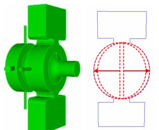
Figure 1: Interior surfaces of the LCLS RF photocathode gun.
