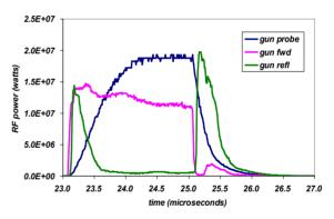
Figure 6: The RF power as measured using a peak power analyzer using calibrations for probes, couplers and cables. See Figure 4 for the location of measurements in RF circuit.
