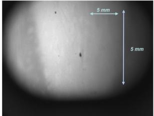
Figure 10: White light image of the cathode area as viewed and illuminated through the grazing-incidence laser ports.
