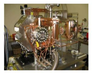
Figure 3: Gun1 and solenoid assembly in the SLAC vacuum lab.
