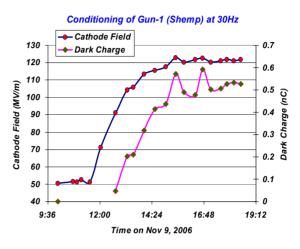
Figure 5: The cathode field and dark charge while conditioning to high power.
