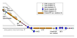
Figure 1: Layout of *LCLS* injector from gun to BC1. The off-axis injector is in a separate enclosure from the linac.
