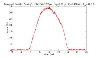
Figure 3: Temporal dist. of 34-A  $e^-$  beam measured with the transverse RF deflector upstream of BC1 ( $\sigma_t \approx 2.0$  ps).
