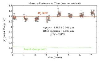
Figure 6: Hor. projected emittance measured over 8 hours.
